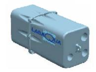
✓ Sampling rate, Rs : "amount of contaminant accumulated per unit time". Rs (D, geometry, <u>turbulence</u>, temperature, biofilm)
